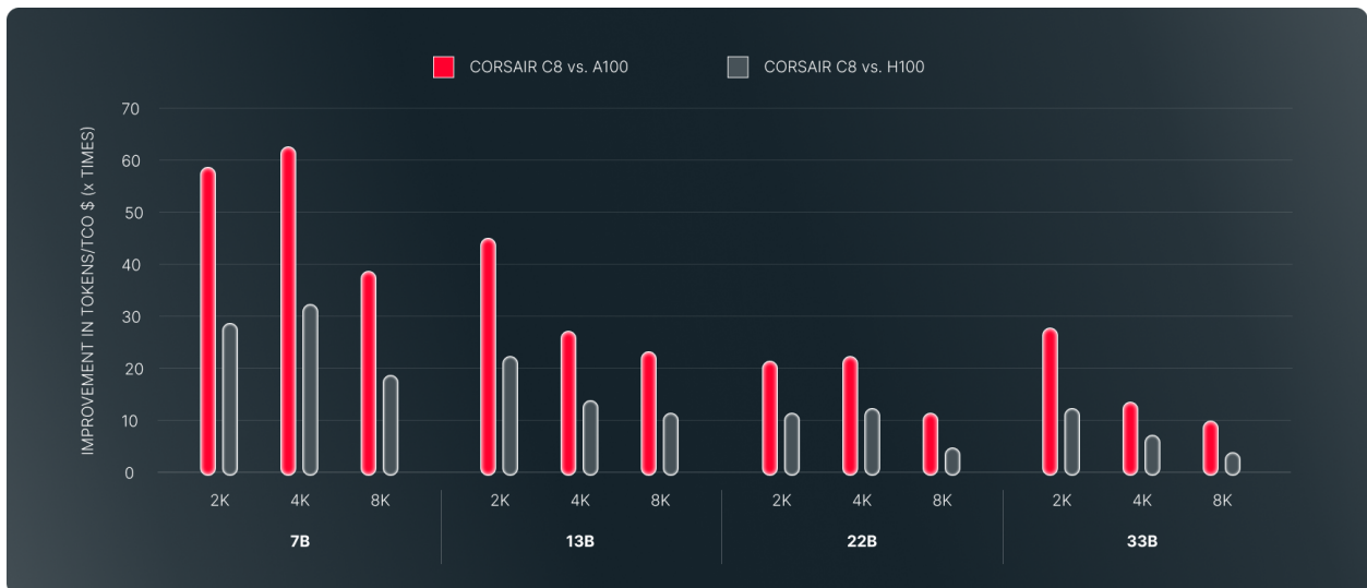
TCO improvement with Corsair for LLMs of different sizes and different context lengths. Beam search decoding with beam=4 and 75:25 input:output tokens is assumed. Results are preliminary and subject to change.
